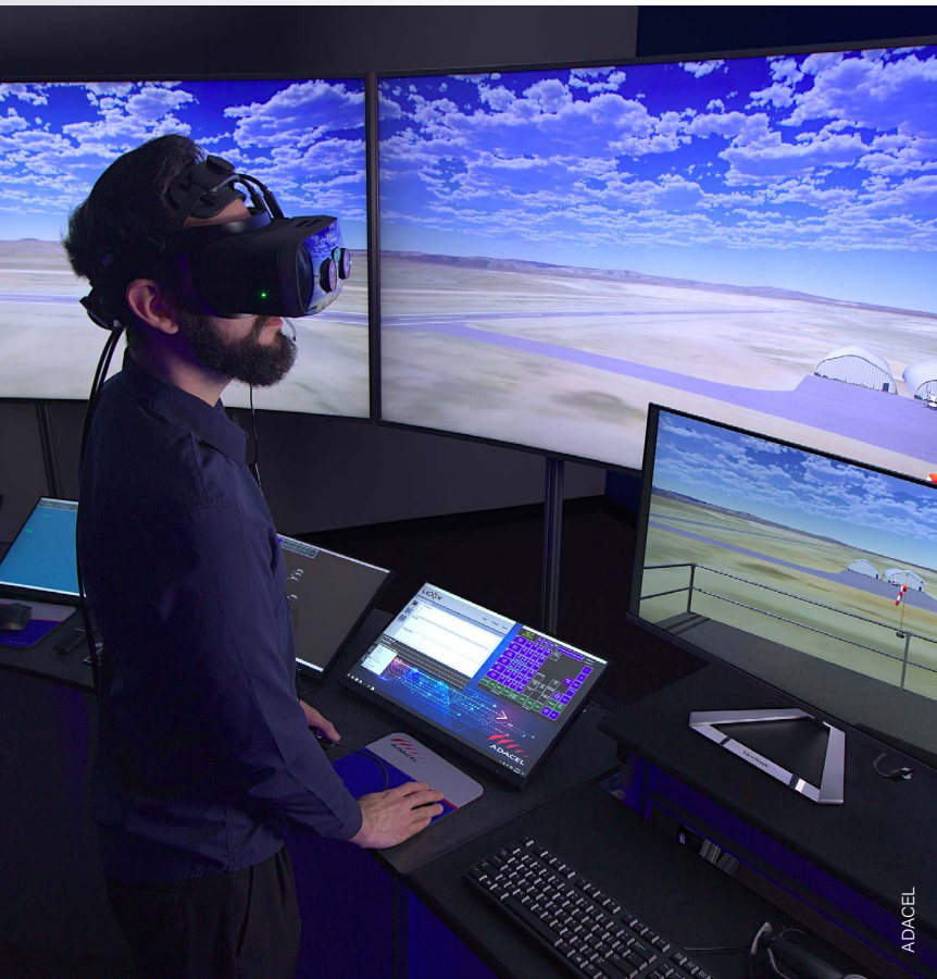
▲ Adacel's MaxSim — 3 Screen Tower Simulation System (TSS)
