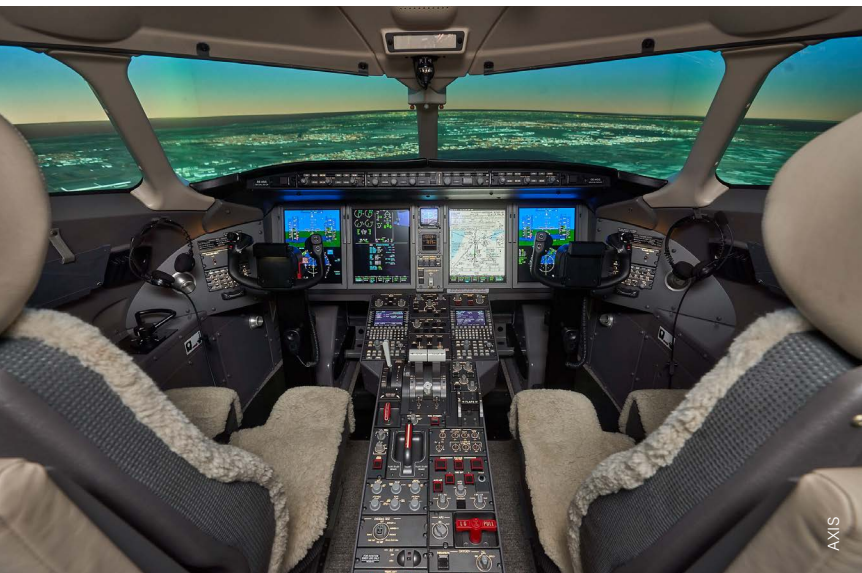
▲ An AXIS Level-D CL350 full flight simulator cockpit.
